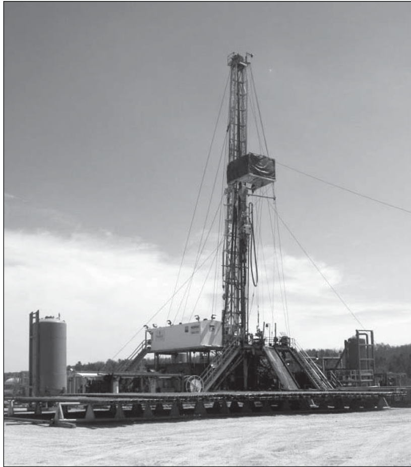
Figure 3.1. A Marcellus Shale drilling rig outside Towanda, Pennsylvania. A drilling rig stays on site for only the duration of the drilling of the well or wells, and can be assembled or disassembled in the course of a few days. The drilling operation itself lasts several weeks for each well; several wells could be drilled on the same well pad, so the duration that a drilling rig stays on site can vary.
