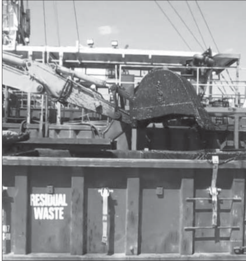
Figure 2.1. A waste container on a drill pad being filled with drill cuttings—finely ground rock pieces removed from the well bore during drilling—near Towanda, Pennsylvania.
