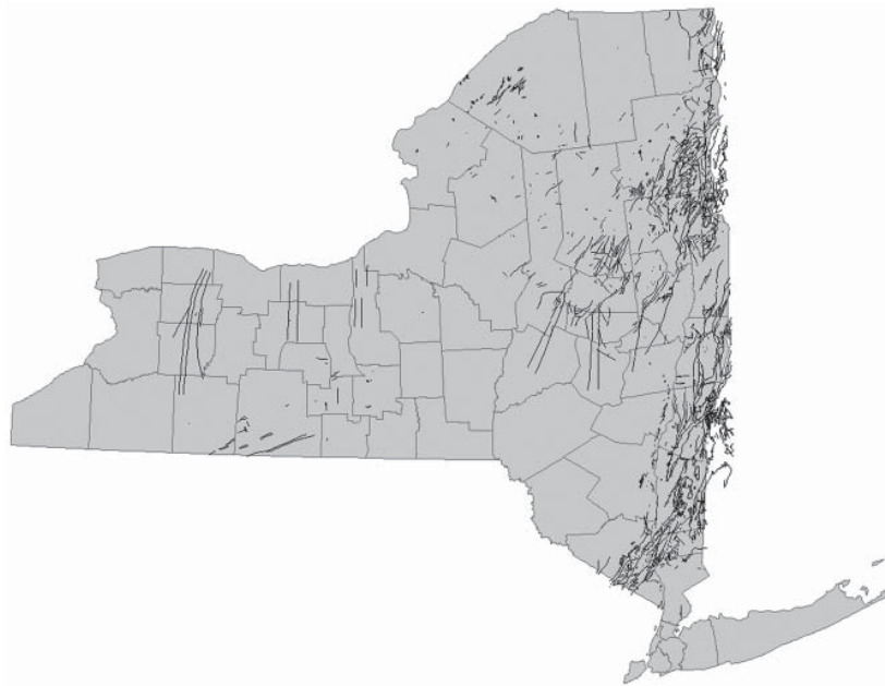
Figure 2.4. The location of active and inactive faults within New York State. Lines denote the location of faults, usually found beneath the surface. Note the high concentration of faults near the eastern state boundary.
