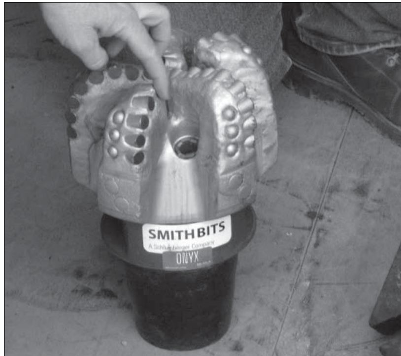
Figure 3.8. A fixed cutter drill bit. Different kinds of bits are used for different parts of the operation, and certain bit types are more effective for drilling in different kinds of rock.
