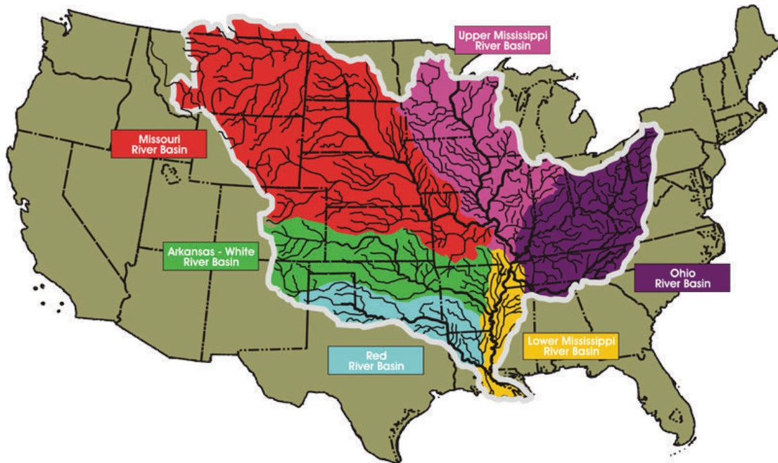
Figure 3: The Mississippi River watershed is comprised of the Mississippi River and many tributary streams that flow across more than 30 states. Here the four largest tributaries are shown: the Missouri River, the Arkansas River, the Red River and the Ohio River. All rainfall within this watershed flows to the ocean at the mouth of the Mississippi River, just downstream of the city of New Orleans (US Army map).
