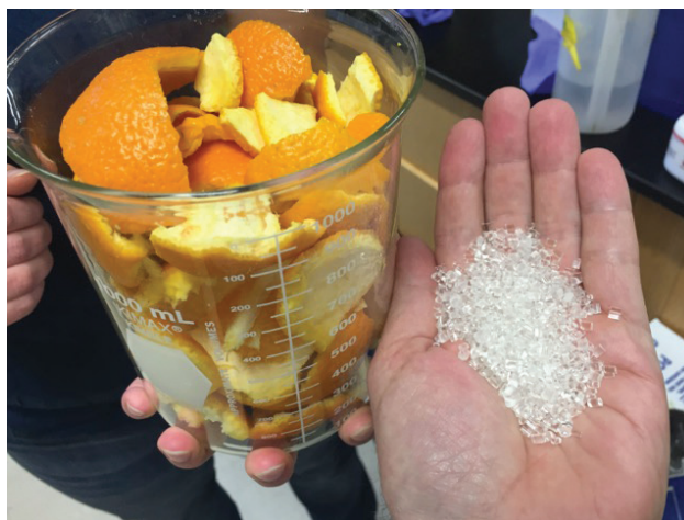
Figure 7.13: Polymers created using carbon dioxide and limonene oxide derived from orange peels.
